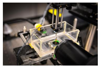
Duke and Stanford Universities' researchers have developed a new clip-on device that upgrades a standard two-dimensional (2D) ultrasound with three-dimensional (3D) imaging capabilities. The device features a \$10 microchip that is common to smartphones and 3D-printed materials and is designed to allow a 2D ultrasound machine to capture 3D images of infants' brains while the baby is held in a parent's arms.
