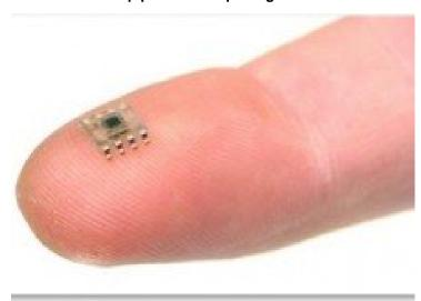
A team of researchers at the Fraunhofer Institute for Cell Therapy & Immunology, Germany, have devised a new lab-on-a-chip platform for detecting microorganisms in individual samples.
