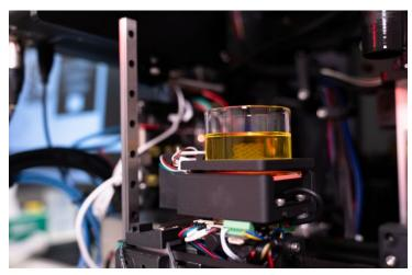
Biomedical engineers from the University of Melbourne, Australia have invented a 3D printing system, or bioprinter, capable of fabricating structures that closely mimic the diverse tissues in the human body, from soft brain tissue to harder materials like cartilage and bone.
