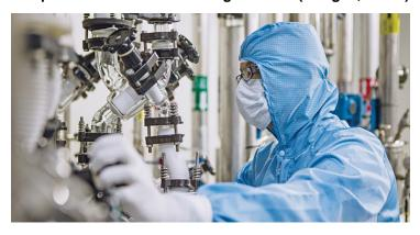
WuXi STA, a WuXi AppTec company, has opened another high-potency API (HPAPI) plant at its Changzhou site (Jiangsu, China). The new plant will meet the growing demand for high-potency API process R&D and manufacturing services and consists of reactors from 250 L to 3,000 L, prep-HPLC systems, a 10 m2 tray lyophilizer, as well as flow chemistry and milling technologies.
