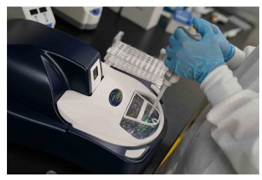
Traditional LAL test methods, which include the 96-well plate and gel clot, are labor-intensive, prone to errors, and may fall short of today's data integrity needs. Overall, these traditional methods are time consuming and leave a lot of room for improvement in terms of the analyst's hands-on time and ergonomics.
