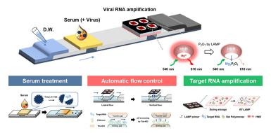
Researchers from Gwangju Institute of Science and Technology in Korea have developed a simple and low-cost diagnostic platform—a *lab-on-paper* strip—that can readily detect the specific RNA of these viruses from a small blood sample.
