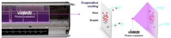
South Korea based Seoul Viosys, is promoting new Violeds technology solution, the world's first ultraviolet LED technology proven to sterilize new coronaviruses, for air conditioning and heating systems.
