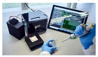
A team of researchers at the National University of Singapore (NUS) has developed a portable COVID-19 micro-PCR diagnostic system – called Epidax – that enables rapid and accurate on-site screening of infectious diseases and significantly reduces the time required to analyse patient samples.
