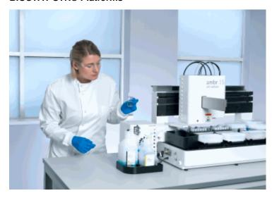
Caption: ambr® 15 cell culture system with ambr® analysis module showing BioPAT® Spectro port; to which a probe for Raman spectrometer is connected
