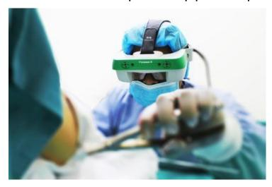
Foresee-X is a set of smart surgical glasses with functionality based on augmented reality (AR) and mixed reality technologies. This device was developed by SURGLASSES, also known as Taiwan Main Orthopaedic Biotechnology Co. Ltd., and has received IEC60601-1-2 and ISO 13485 certifications. It is designed to bring a higher level of support to surgical procedures for trauma cases.
