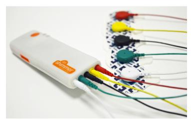
Shimmer Research, a global leader in wearable technology for research applications, on 4 Nov 2019, announced that ECGmd – its five-wire, four-lead holter monitor electrocardiograph (ECG) – is now a CE certified, Class IIa medical device under the Medical Device Directive (93/42/EEC).
