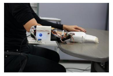
The Biological Systems Engineering Lab at Hiroshima University, Japan has developed a new 3D printed prosthetic hand combined with a computer interface, which is their cheapest, lightest model that is more reactive to motion intent than before. Previous generations of their prosthetic hands have been made of metal, which is heavy and expensive to make.
