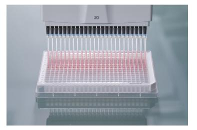
With their 16 and 24 channels, the new mechanical multichannel pipettes Eppendorf Research plus and the new electronic multichannel pipettes Eppendorf Xplorer plus can now tackle entire columns and rows of a 384-well plate in one single step. Up to 24 reactions may thus be started and stopped simultaneously. An entire plate can be managed manually within the space of a minute. In this way, the user will save time while at the same time improving the reproducibility of their results.
