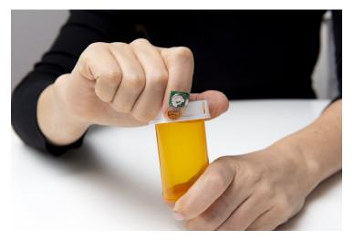
In new research IBM team details a first-of-a-kind "fingernail sensor" prototype to help monitor human health. The wearable, wireless device continuously measures how a person's fingernail bends and moves, which is a key indicator of grip strength.
